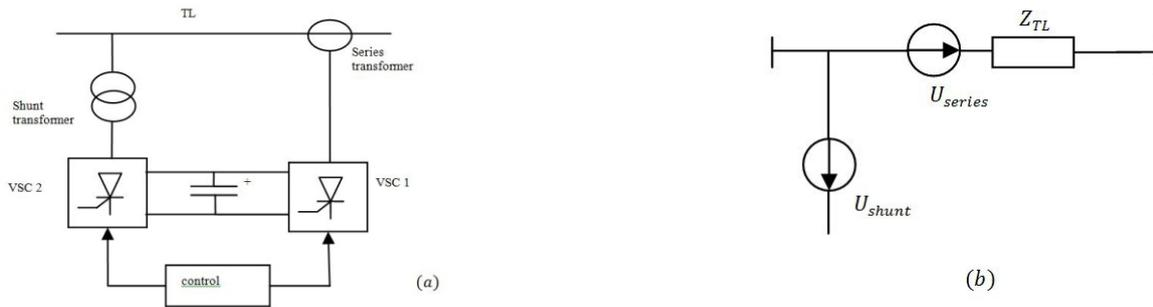
Figure 2: (a) Single Line Structure of UPFC; and (b) Impedance Diagram of Connection of UPFC to TL.
