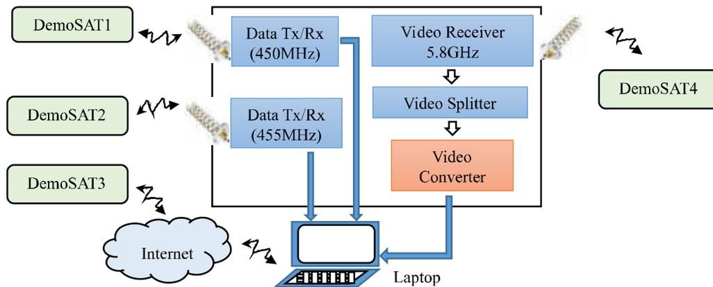
Figure 2: Block Diagram of Ground Station
