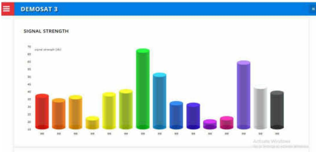
Figure 14: Data visualization of signal strength reading using SIM 800
