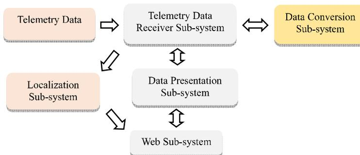
Figure 1: Block Diagram of the Ground Station for Telemetry Data
