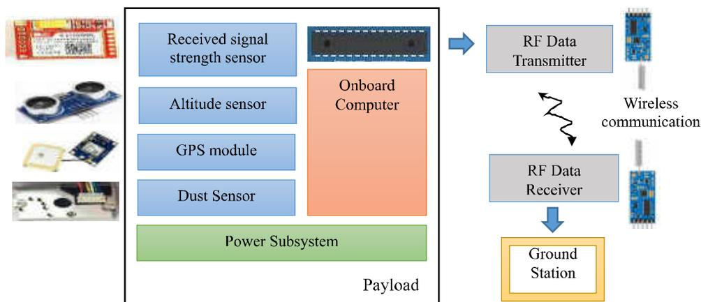
Figure 4: Block diagram of Earth Habitability Monitoring Satellite
