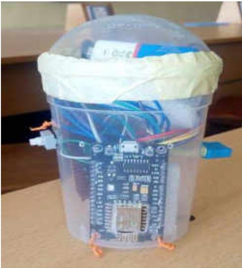
Figure 8: Initial packaging of DemoSAT-I
