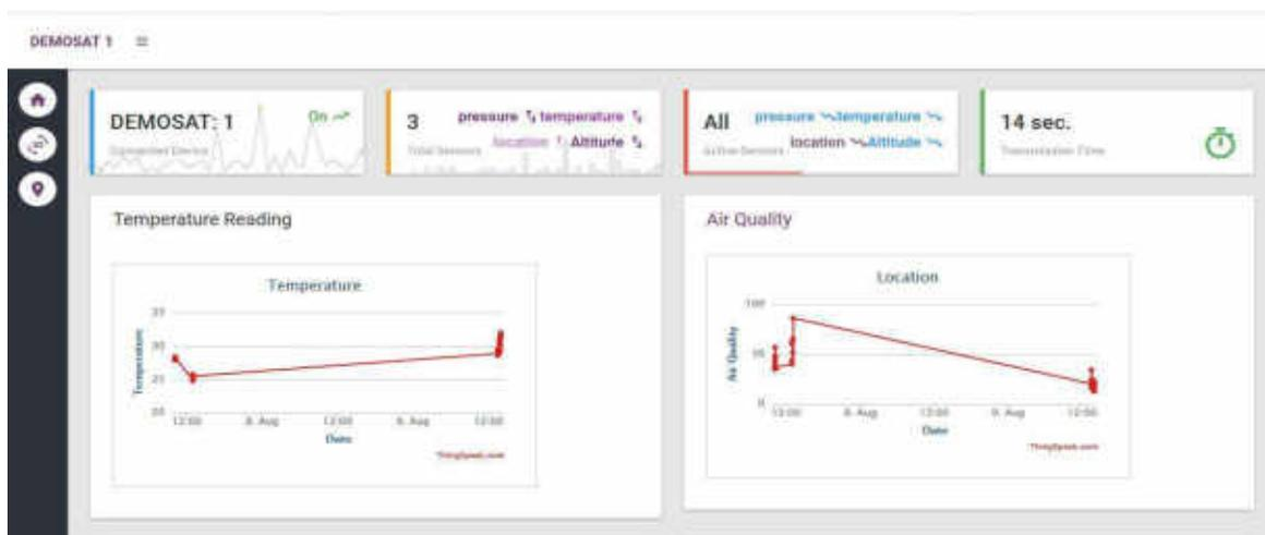
Figure 12: Temperature reading using DHT11 and air quality reading using MQ135.
