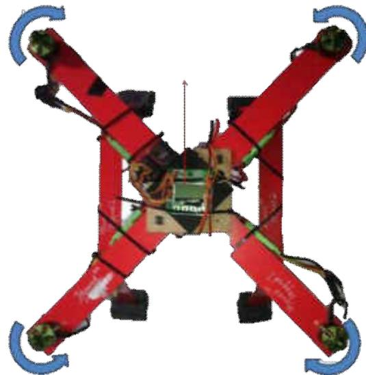
Figure 7: Propeller rotational direction
