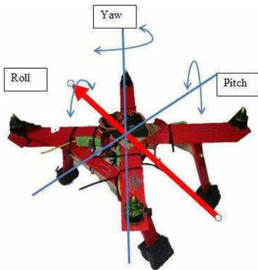
Figure 6: Roll, Pitch and Yaw axes
