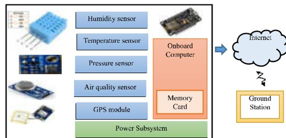
Figure 3: Block diagram of Environment Monitoring Demonstration Satellite
