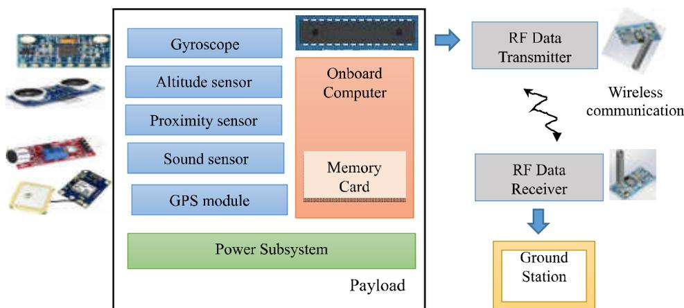
Figure 5: Block diagram of Altitude and Orbit Monitoring Satellite
