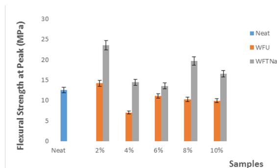
Figure 3. Variation of flexural strength at peak of the developed composite and the neat samples
