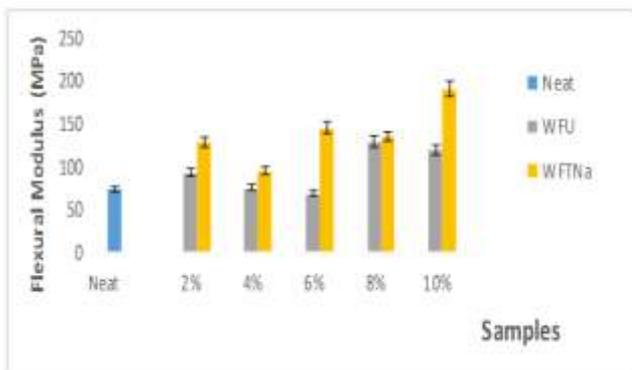
Figure 5. Variation of flexural modulus of the developed samples
