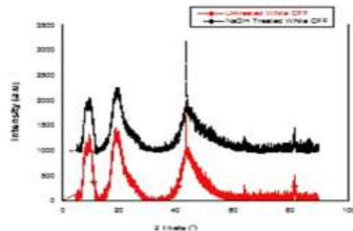
Figure 6. XRD result of untreated white CFF and with NaOH
