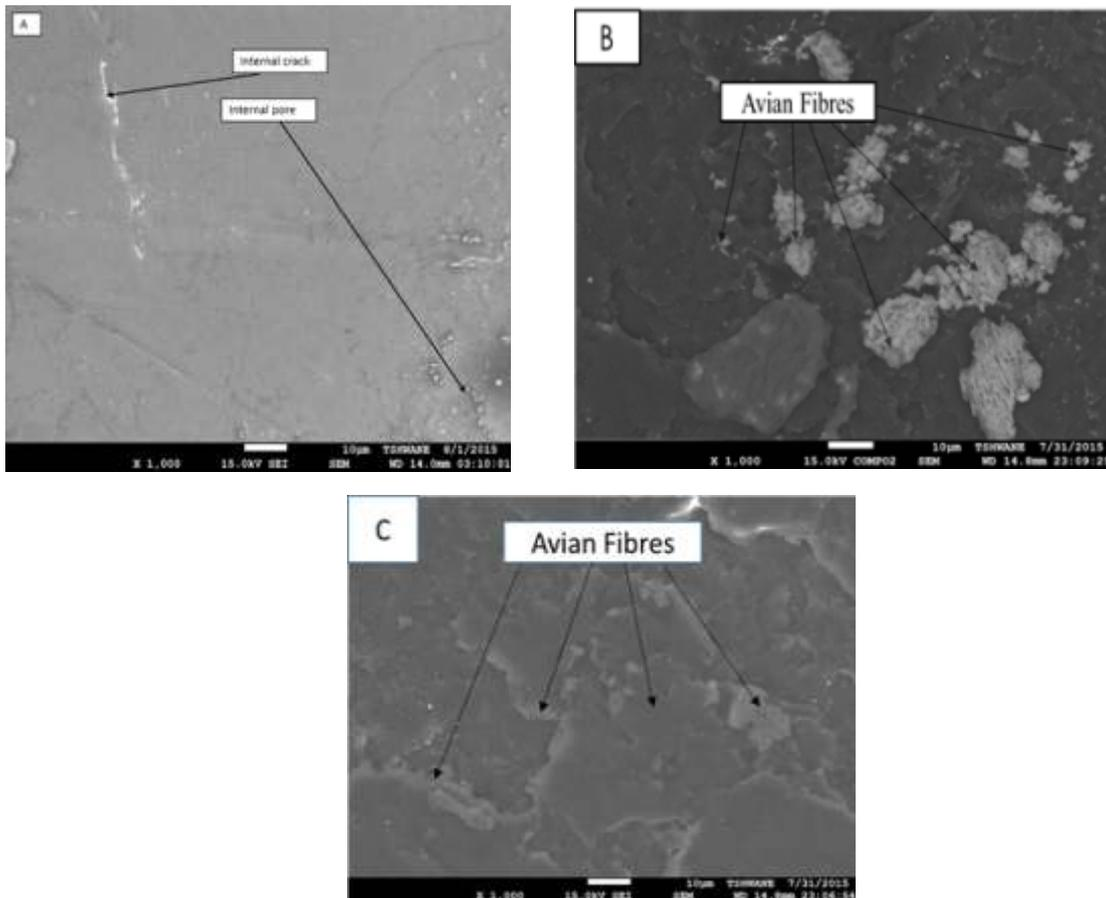
Figure 8. SEM image of the neat sample (A), (B); HDPE reinforced with 10 wt % untreated white CFF and C; HDPE reinforced with 10 wt % NaOH treated white CFF
