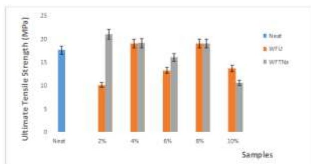
Figure 2. Ultimate tensile strength of the composites and the neat sample
