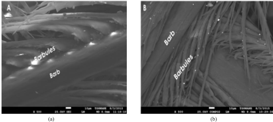
Figure 7. SEM image of untreated white CFF (A) and NaOH treated white CFF (B).
