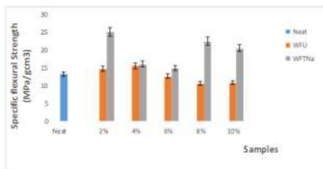
Figure 4. Variation of specific flexural strength of the developed samples
