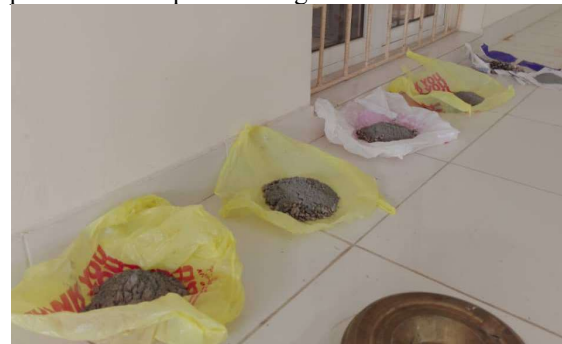
Figure 1: batching of constituents for AMBT
