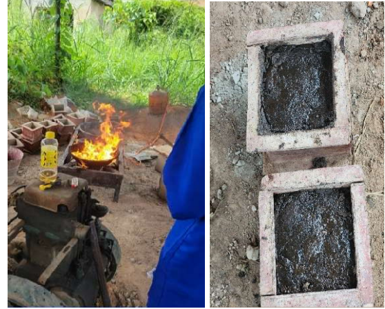
Figure 2: Casting of LDPE Based Concrete
