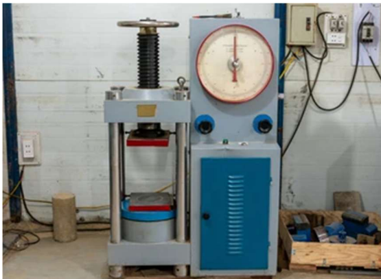
Figure 4: Concrete compression testing machine
