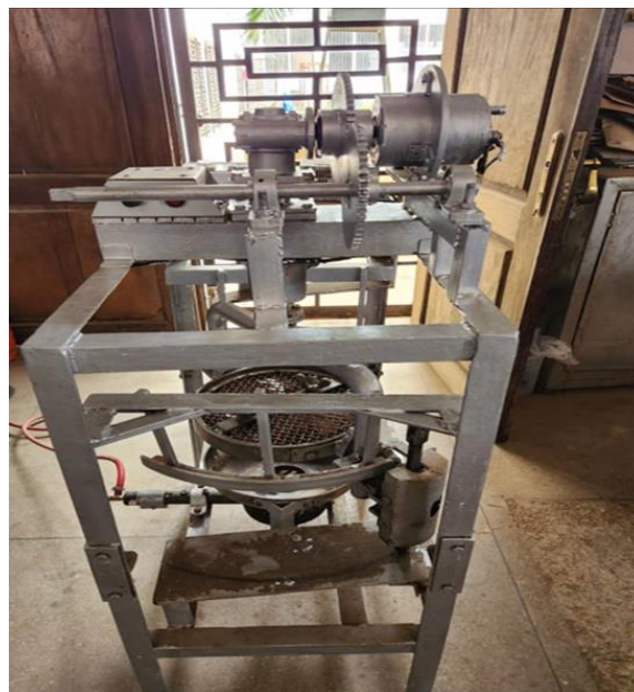
Plate 1: Front View of the Developed Meat Roasting Machine
