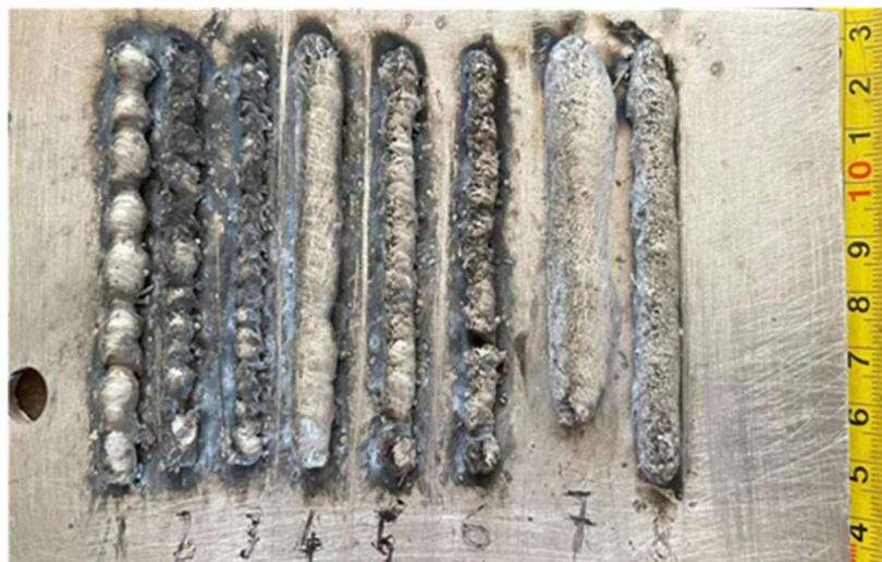
Figure 2: AA5356 single tracks deposited via WAAM-GMAW without argon shielding gas, showing poor surface finish and compromised structural integrity.
