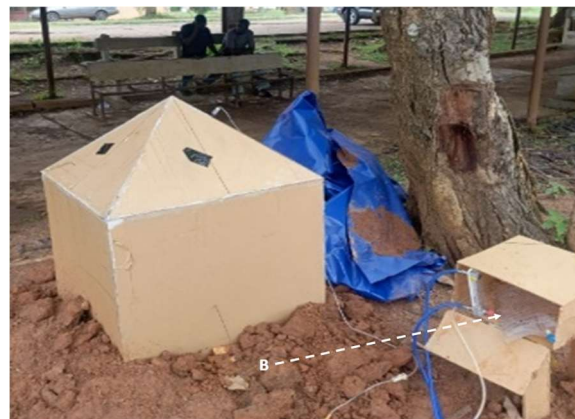
Plate 2: The Experimental Setup Showing the Termireactor with Gas Collection Bag, B.
