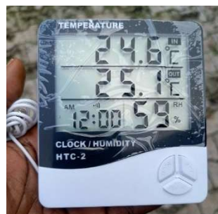
Plate 3: Photograph of a Digital Thermo-hygrograph for Measuring Temperature and Relative Humidity
