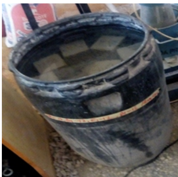
Plate 4: Concrete cubes in curing tank
