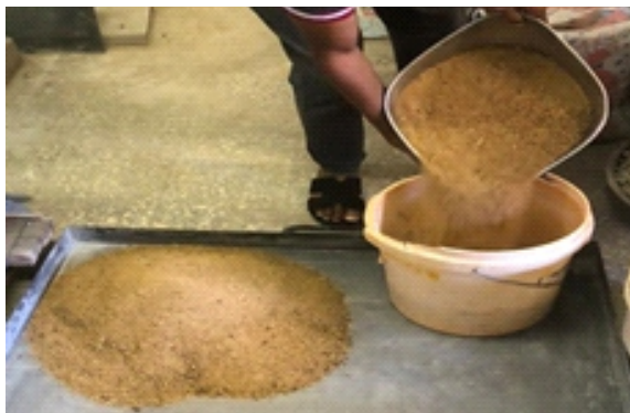
Plate 1(a): Batching of fine aggregate
