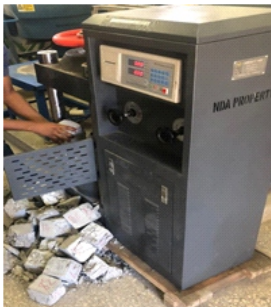
Plate 5: Testing of compressive strength
