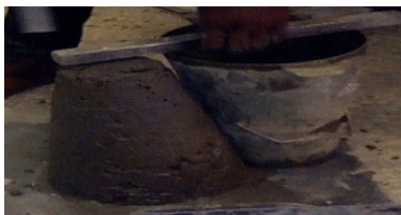
Plate 3: Slump test sample
