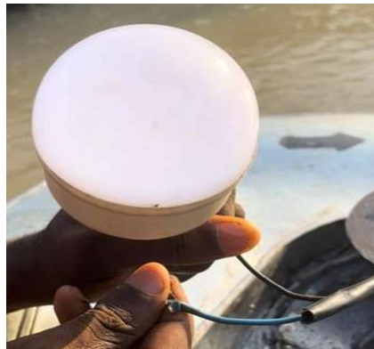
Figure 16. Powering a 60 W light bulb using the turbine-driven alternator
