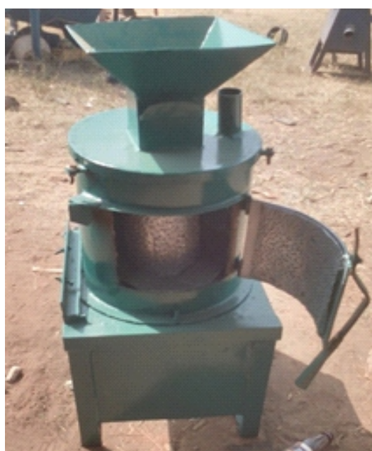
(b) Peeling machine showing internal peeling drum
