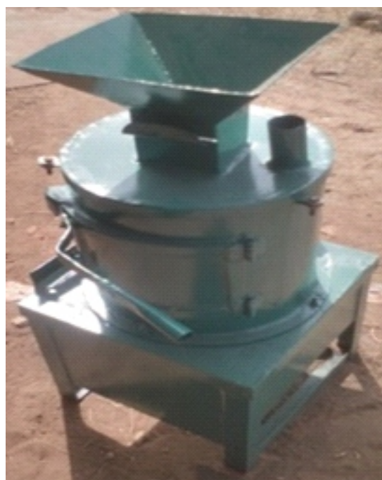
Figure 3: (a) The assembled peeling machine
