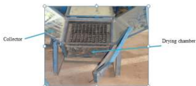
Figure 2: Front elevation of the solar dryer
