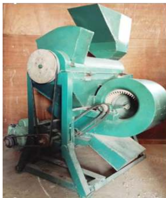
Figure 1: The fabricated maize sheller (Soyoye and Tehinse, 2020)
